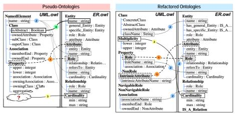
Fig. 4. COMA++ mapping between pseudo-ontologies and refactored ontologies
