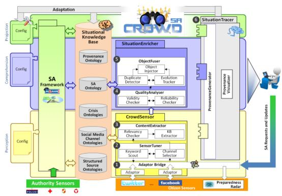
Figure 2: Overall System Architecture
